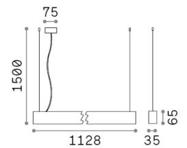
Net weight1.82 kgInsulation classIProtection indexIP20ComplianceCEOperating temperature $0^{\circ} \sim +40 \, ^{\circ}\text{C}$
