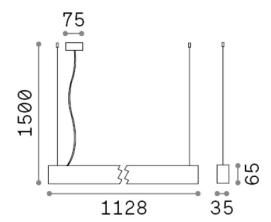
Net weight 1.82 kg Insulation class Ī **Protection index** IP20 Compliance CE Operating temperature 0° ~ +40 °C
