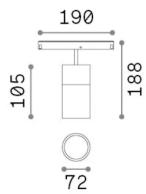
Net weight0.8 kgInsulation classIIIProtection indexIP20ComplianceCEOperating temperature $0^{\circ} \sim +40 \, ^{\circ}\text{C}$
