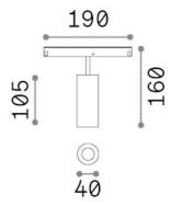
Net weight0.2 kgInsulation classIIIProtection indexIP20ComplianceCEOperating temperature $0^{\circ} \sim +40 \, ^{\circ}\text{C}$
